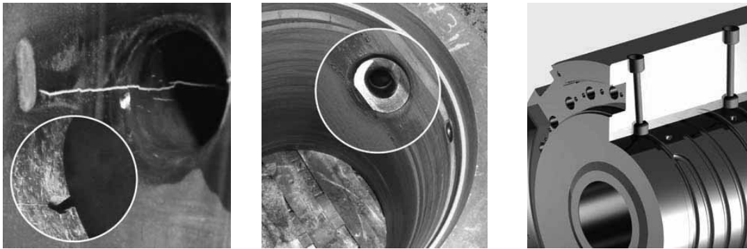
Figure 6. Container mantle before and after installing AP-system
