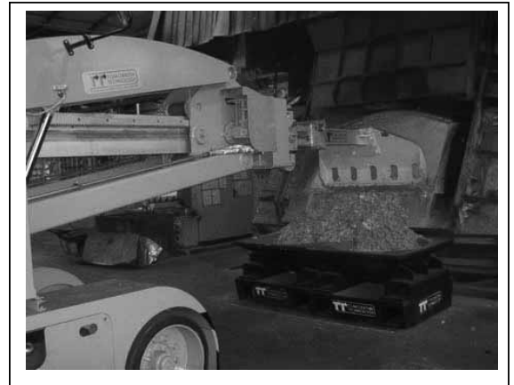
12. T.T. MFTV during de-drossing operation
