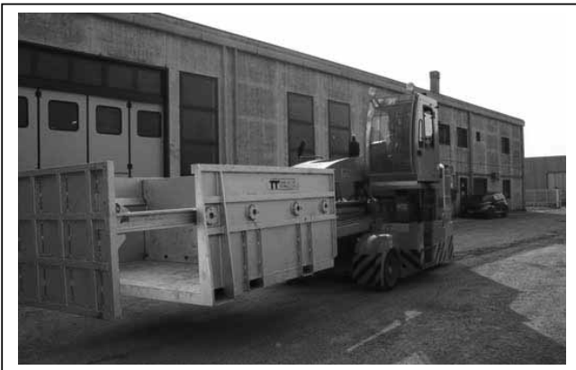
5. T.T. Multifunctional Furnace Tending Vehicle (MFTV)
