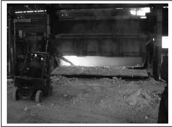
3. Skimming operation by forklift
