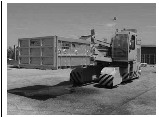
7. T.T. Multifunctional Furnace Tending Vehicle (MFTV) 8 tons net capacity
