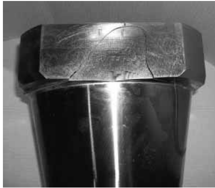
Figure 7. Damage on press stem
