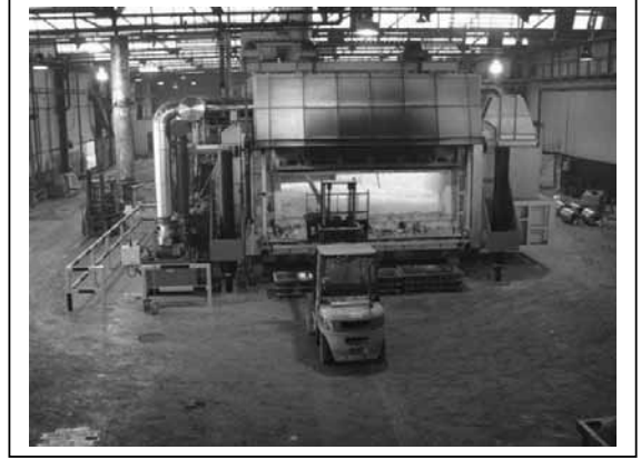
2. Skimming operation by forklift
