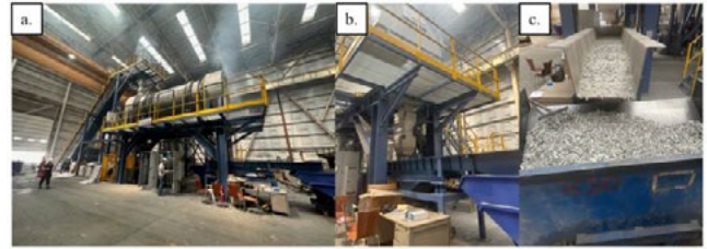
Figure 3. Delacquering Process; a) Delacquering Rotary Kiln System of ASAS, b) Outlet Side of the System, c) Delacquered Scraps
