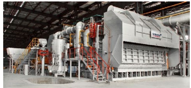
Fig. 1: Twin-chamber melting furnace for recycling aluminum scrap
