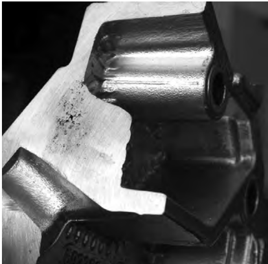
Picture 10a: Cut through a high-mess section of a casting part. You can see shrinkage holes which are connected with the surface and draws.
