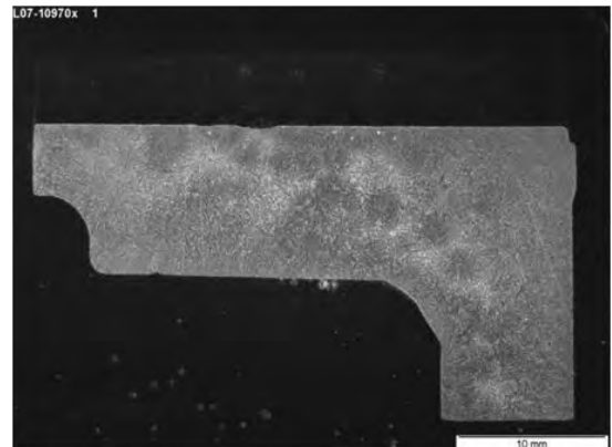
Picture 7b: A cut through the line in picture 9 shows the draws.
