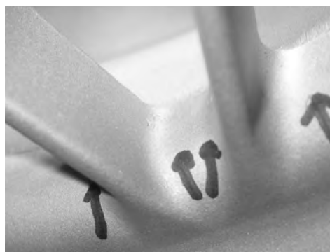
Picture 16: Application of a master alloy at an aluminium rim. The spokes and the rim base often have shrinkage holes, which are partly extend to the surface (the arrows hint at very small open sections in the casting part).
