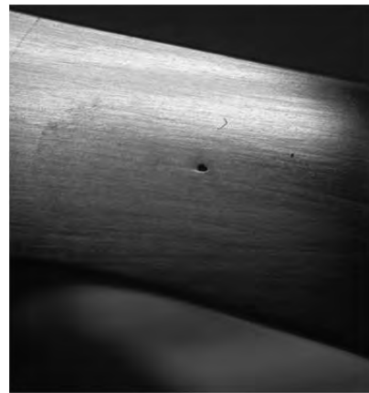
Picture 13b: The cross section shows a little shrinkage hole or a pore which does not harm the functionality or strength of the casting part.
