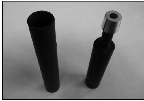
Picture 8. Coated tool-couple with Al-specimen.
