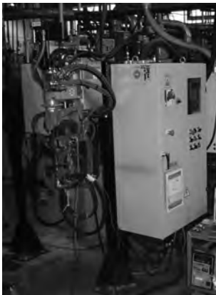
Figure 13. ARO Electric Servo-Gun with MFDC Power Supply
