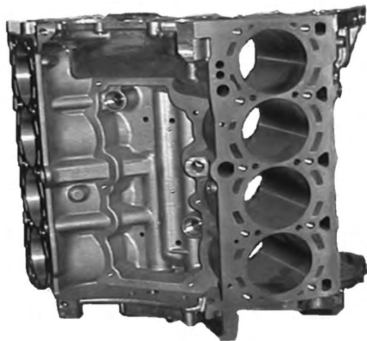
Picture 18: Engine block casted with an AlSi17Cu4Ni. The scrap rate could be highly reduced by the addition of nano structured oxides. 1kg / t of the master alloy PROBAT-FLUSS MIKRO 100 made up the charge.
