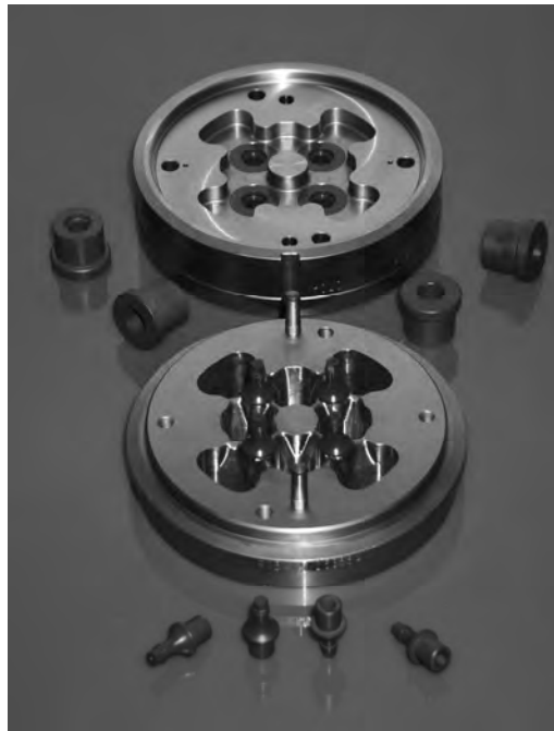
Picture 10. 4-cavity round tube die with CVD coated inserts
