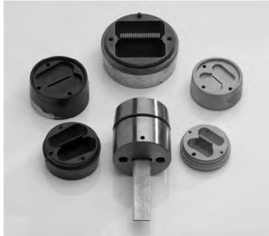
Picture 1. CVD coated extrusion dies for heat exchanger profiles.
