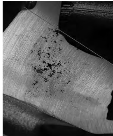
Picture 10b: The blow-up of the cross section shows the branchy structure of the shrinkage holes, its opening to the surface and the clear draws (deviation from the red line).
