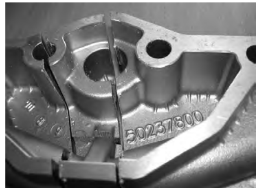
Picture 8b: A smooth surface could be obtained by treating the melt with PROBAT-FLUSS MIKRO.
