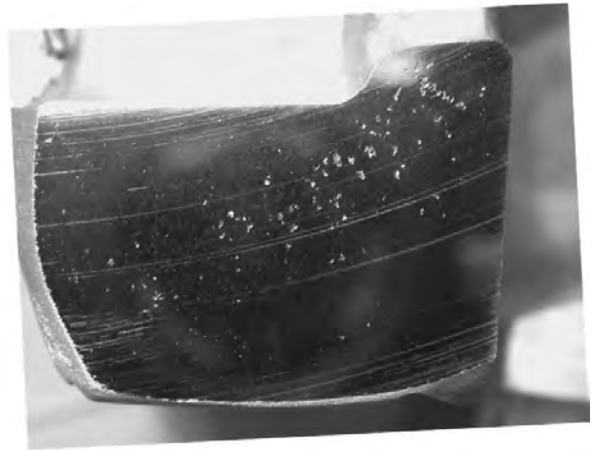
Picture 9b: After the addition of nano structured oxides by 1 kg/t of the master alloy, the volume contraction is compensated and draws are prevented.
