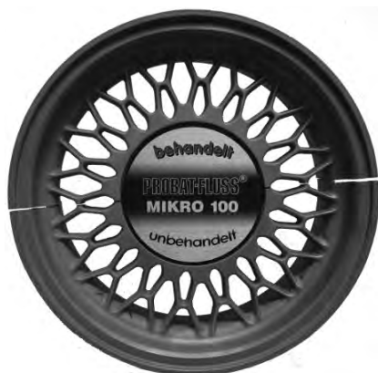
Picture 15: Rim with a lot of spokes. This wheel consists of one wheel half without any treatment with a lot of defects (picture 16) and another half treated with nano structured oxides. This half does not show any x-ray scrap.
