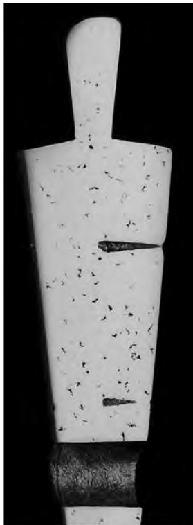
Picture 6a: Wedge test piece with impeded feeding. Cavities with an edged structure can be observed.
