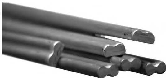
Picture 4: Master alloy with nano structured oxides (trade name: PROBAT-FLUSS MIKRO 100).
